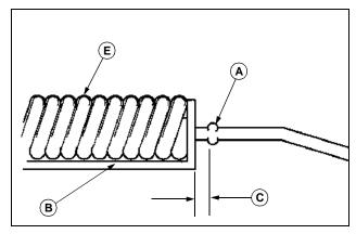
3. Measure distance from inside of brake rod stop tabs (A) to outside of compression spring bracket (B) (located below foot tread area on left-hand side of transmission). Distance (C) should be 2-10 mm (0.08-0.40 in).
